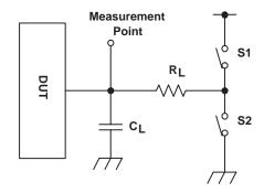
**Figure 5. PFD Output Test Conditions**
