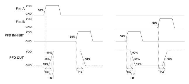
Figure 4. PFD Output Voltage Waveform Table 4. PFD Output Test Conditions
